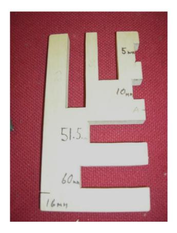
Cutting the wood to exactly the right length by using this jig means that you don't then have to use an end mill to trim the wood that pokes out beyond the end of the brass inserts.
