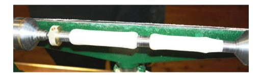
The finished profile can now be sanded down using your preferred abrasives. Make sure you don't remove the details with excessive sanding. Bob used Scotchbrite and a Hermes 180 grit sanding pad.
