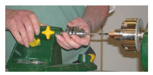
Use a slow speed for drilling, to prevent the wood from overheating and potentially splitting.
